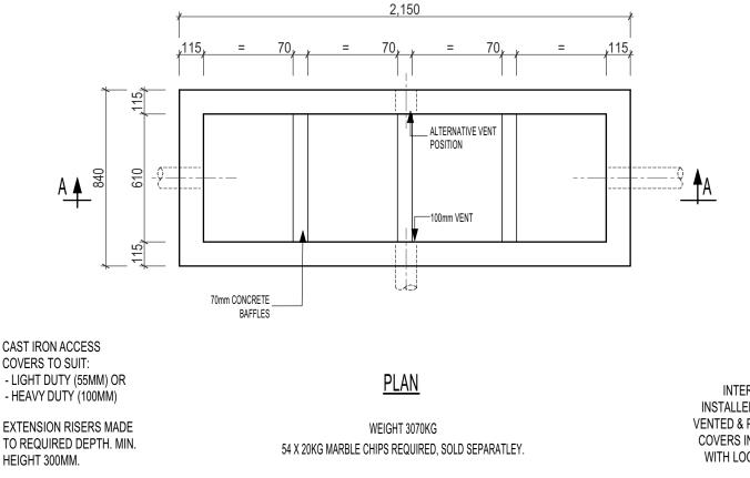
INTERCEPTOR TO BE INSTALLED, CONNECTED, VENTED & PROVIDED WITH COVERS IN ACCORDANCE WITH LOCAL AUTHORITY.
