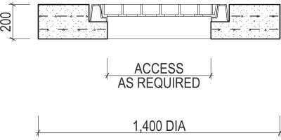
COVER LOCATION & SIZE SPECIFIED MUST BE SUITABLE TO ACCOMODATE PUMP REMOVAL
