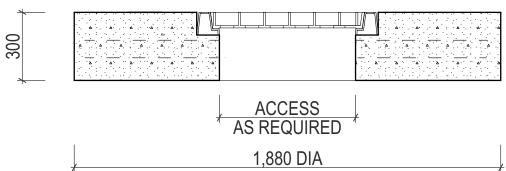
**COVER LOCATION & SIZE** SPECIFIED MUST BE SUITABLE TO ACCOMODATE PUMP **REMOVAL**
