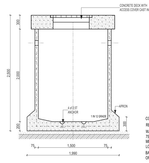
CONCRETE 40MPa 28 days. REINFORCEMENT
